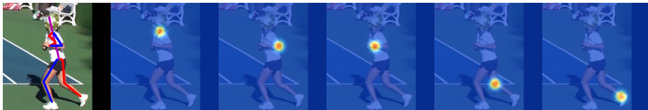
Fig. 2. Example output produced by our network. On the left we see the final pose estimate provided by the max activations across each heatmap. On the right we show sample heatmaps. (From left to right: neck, left elbow, left wrist, right knee, right ankle)
